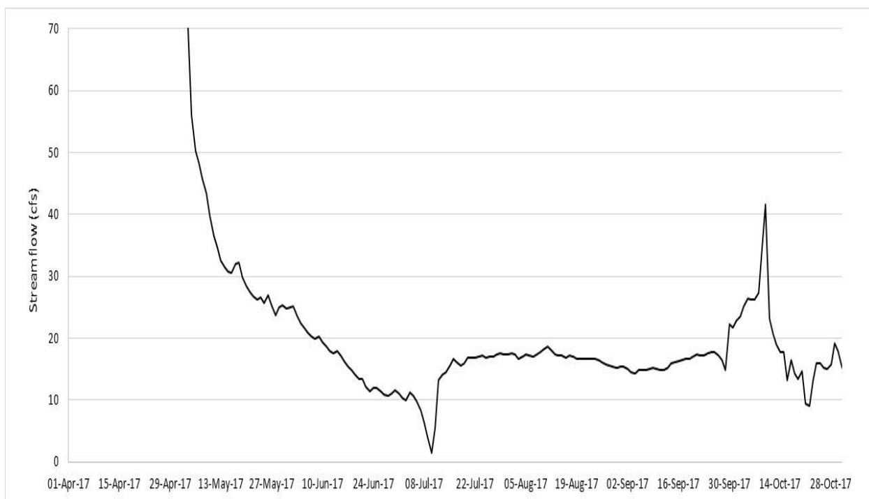
Figure 7. Mean daily stream flow at the SCVWD Edendale gage (in the urban area downstream of Metcalf Percolation Pond) from 1 April through 1 November 2017.
